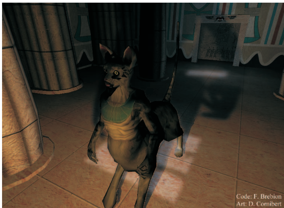
Screen shot taken from the soft shadows demo. This 6,000-triangle temple scene features six lights, two of which are casting spherical soft shadows, and runs at up to 35 fps on a Radeon 9700. The two lights are animated. (See page 578.)
