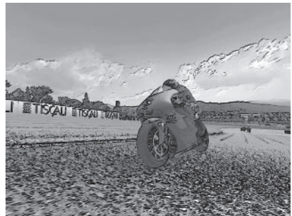
Figure 4: The cartoon shader starts by applying an edge detect filter.
