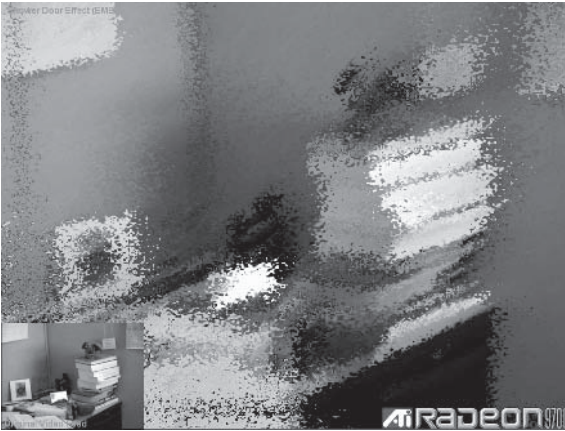
Figure 10: The shower door effect is created by using a noise texture to perturb the normals used in environment mapping.
