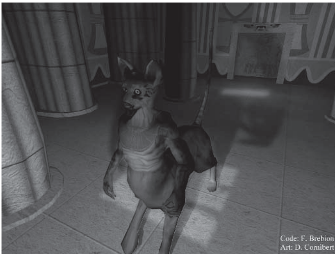
Figure 19: Screen shot taken from the soft shadows demo. This 6,000-triangle temple scene features six lights, two of which are casting spherical soft shadows, and runs at up to 35 fps on a Radeon 9700. The two lights are animated. (See Color Plate 27.)
