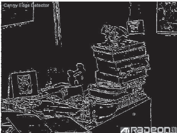
Figure 4: One-pixel-wide edges from the Canny filter
